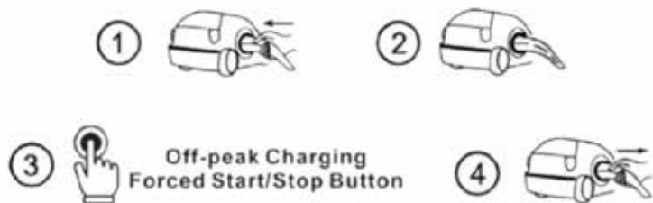
Plug&Charge Mode Operation Diagram
