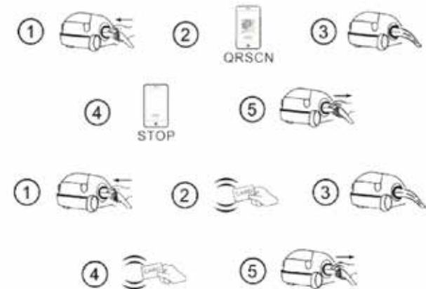
APP/RFID Mode Operation Diagram
