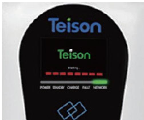
NETWORK Web on, flashing when connect with Internet but dose not connect OCPP. If connect both, the light will on. Light off if does not connect internet.
